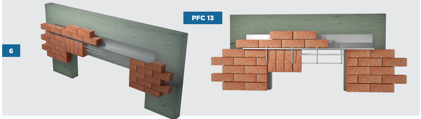
PFC 65/2V EXTENDED SUPPROTING CONSOLE WITH 2 MODULES FRONT OF THE SHUTTER CASE - VISIBLE
