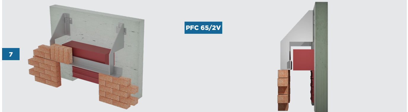
PFC 65/2V EXTENDED SUPPROTING CONSOLE WITH 2 MODULES FRONT OF THE SHUTTER CASE - VISIBLE
