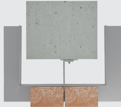
PFC 64/1 PILLAR SUPPORT CONSOLE WITH 1 MODULE - CLOSING THE FACADE WALL-FACE
