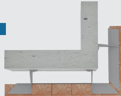
PFC 67/2-J45 BEVEL CORNER SUPPORTING CONSOLE- CORNER WITH CLOSED GAP
