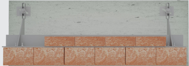
PFC 26/2V HANGING PROFILE CONSOLE WITH 2 MODULES AND PREPRODUCED HORIZONTAL CONCRETE BRIDGING
