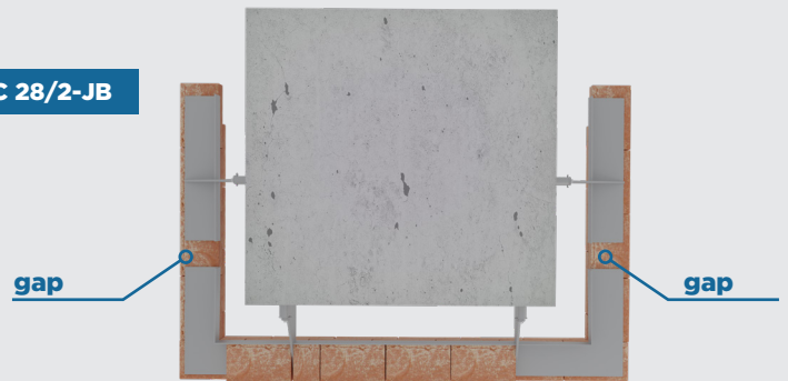
PFC 28/2-JB 2 CORNER PLATED CONSOLE WITH 2 MODULES - CORNER AROUND THE PILLAR
