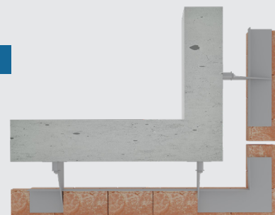
PFC 28/2J CORNER PLATED CONSOLE WITH 2 MODULE - CORNER WITH OPENED GAP
